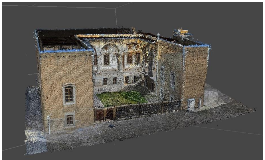
Figure 8. Fatah Chalabi house, Point cloud generation. The model represents the building's surface as a dense collection of points
